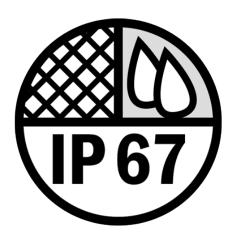
The IP Code, International Protection Marking, sometimes misinterpreted as Ingress Protection Marking, classifies and rates the degree of protection provided against the intrusion (including body parts such as hands and fingers), dust, accidental contact, and water by mechanical casings and electrical enclosures.
