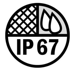
The IP Code, International Protection Marking, sometimes misinterpreted as Ingress Protection Marking, classifies and rates the degree of protection provided against the intrusion (including body parts such as hands and fingers), dust, accidental contact, and water by mechanical casings and electrical enclosures.
